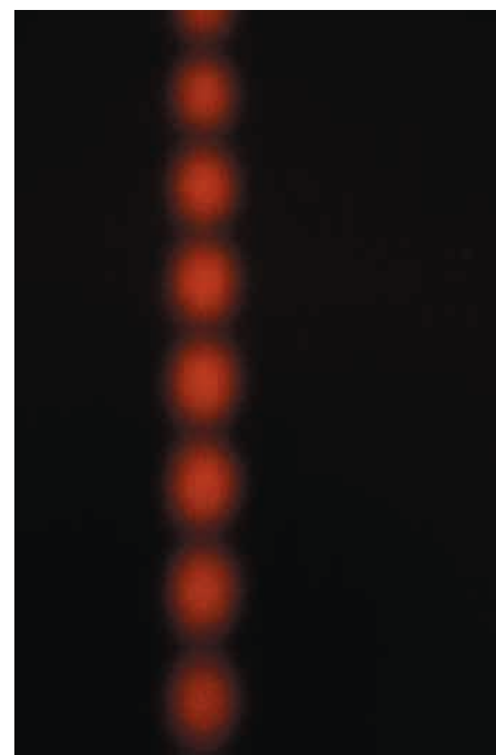
Fig. 35-9 A photograph of the interference pattern produced by the arrangement shown in Fig. 35-8, but with short slits. (The photograph is a front view of part of screen C .) The alternating maxima and minima are called interference fringes (because they resemble the decorative fringe sometimes used on clothing and rugs). (Jearl Walker)
