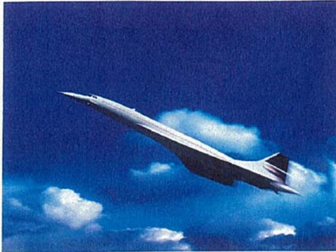
Fig. 18-9 When a Concorde flew faster than the speed of sound, thermal expansion due to the rubbing by passing air increased the aircraft's length by about 12.5 cm.
